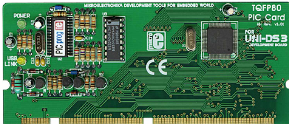
PIC 80-pin Card for UNI-DS3 For Microchip PIC MCU's. USB 2.0 programmer on-board. Comes with P18F8520.
