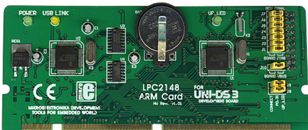
ARM Card for UNI-DS3 For new ARM MCU's. USB 2.0 programmer on-board. Comes with LPC2148.
