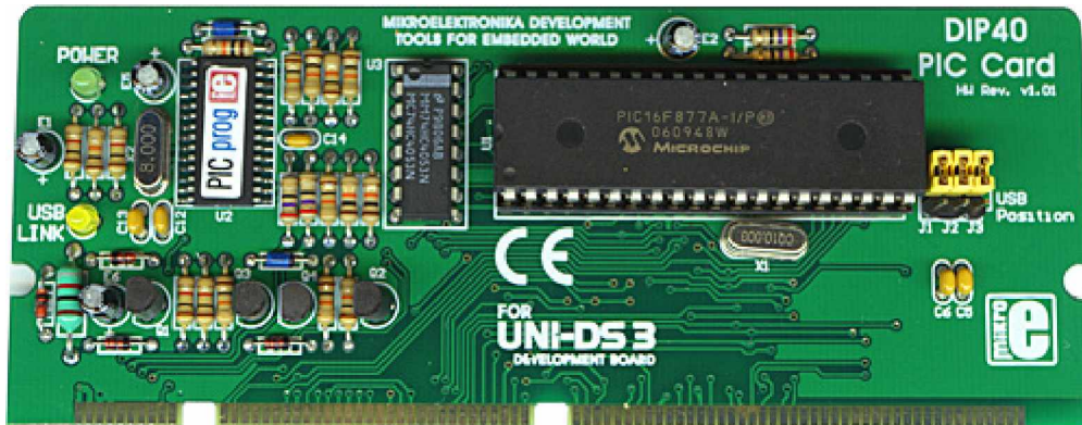
PIC 40-pin Card for UNI-DS3 For Microchip PIC MCU's. USB 2.0 programmer on-board. Comes with P16F877A.
