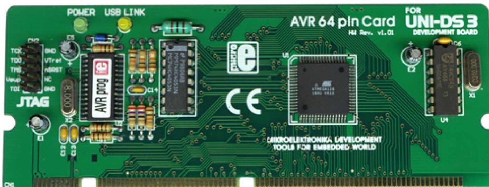
AVR 64-pin Card for UNI-DS3 For Atmel AVR MCU's. USB 2.0 programmer on-board. Comes with ATMEGA128.
