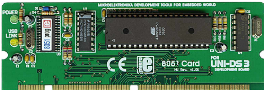
8051 Card for UNI-DS3 For Atmel 8051 MCU's. USB 2.0 programmer on-board. Comes with AT89S8253.
